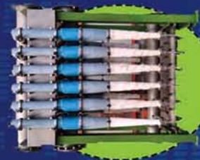
LD Cleaner Used to remove the heavy rejects that density is higher than 1 g/cm 3 , most popular cleaning equipment.
