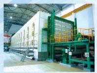
**Double Wire Air Borne Drying Pulp Machine** Trimmed width:2400~6600 mm Machine speed:50~250 m/min Basis weight:600~1200 g/m<sup>2</sup>
