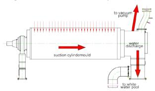
Figure 3 Working Principle of Suction Cylindemould
