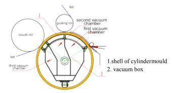
Figure 2 Section View of Suction Cylindermould
