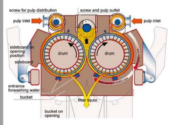
Twin roll press with screw pulp distribution
