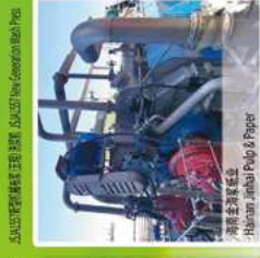
卧式真空洗浆机 Wash Press by Mechanical Drive 竹浆 500T/D 改造项目 For 500T/D bamboo pulp project
